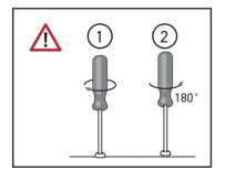
Carefully screw 360° and then unscrew 180° and repeate to remove metal swarf and reduce stress on screws.
